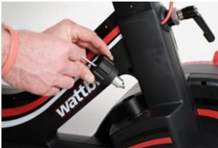
5. Use a 3mm Allen key to remove the 4 long bolts either side of the saddle and handlebar stems. **N.B Keep separate from the other screws as these are a different length.**
