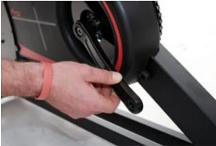
7. Remove 2 x Allen headed bolts on the left hand side using a 4mm Allen key and an 8mm spanner.
