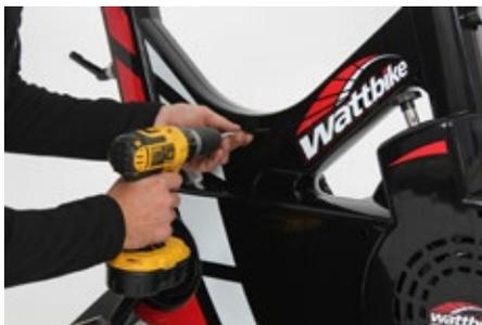
5. Use a 3mm Allen key remove the screw in the column of the magnetic resistance and lift the knob off.
