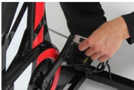
5. Use a 2.5mm Allen key to remove the two Allen headed screws holding the cover to the frame.
