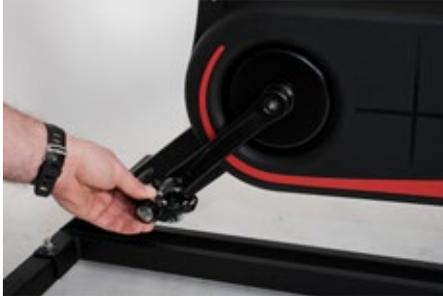
8. Pull the cover away from the bike threading it over the crank and pedal.
