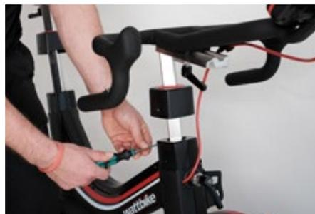
6. Continue to remove the remaining 8 shorter bolts around the cover using a 3mm Allen key.
