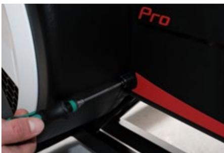
3. Use a 3mm Allen key to remove the 4x Allen headed bolts on the right hand side of the cover in the following order: 1, 2, 3, 4. Ensuring you hold the turbine cover whilst removing. SHOW NUMBERS ON PIC
