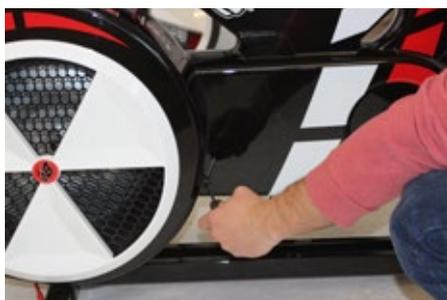
3. Use a cross head screw driver to remove the 4 x 20mm screws attaching the turbine cover on the right hand side of the bike, ensuring you hold the turbine cover whilst removing it.
