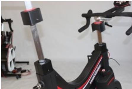
4. Use a 2.5mm Allen key to remove the 4 screws on the step through cover.
