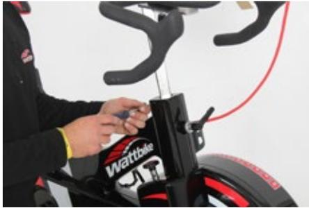
3. Use a 2.5mm Allen key to remove the screw holding the cover to the frame.
