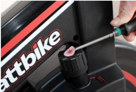
2. Use a 4mm Allen key and insert it in to the middle of the magnetic adjuster dial and unscrew the Allen headed bolt.
