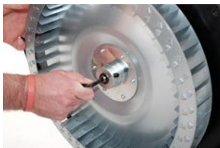
4. Remove the fan wheel. Occasionally the fan wheel can seize to the Axle. A gear puller may be required to help remove the fan wheel.
