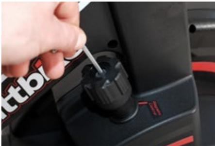
3. Rotate the knob so that magnetic resistance is fully on.
