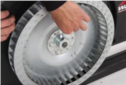
2. Use a 5mm Allen key to remove the bolt securing the fan wheel.
