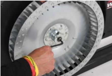
3. Remove the fan wheel. Occasionally the fan wheel can seize to the Axle. A gear puller may be required to help remove the fan wheel.
