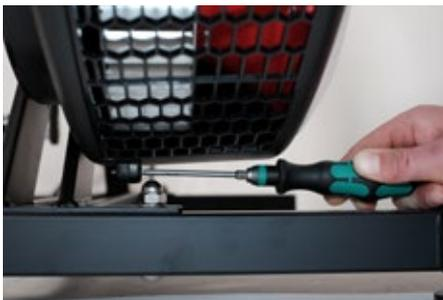
2. Using a 3mm Allen key remove all the screws attaching the turbine cover to the left hand cover
