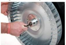
Remove the fan wheel. Occasionally the fan wheel can seize to the Axel. A gear puller may be required to help 4. remove the fan wheel.
