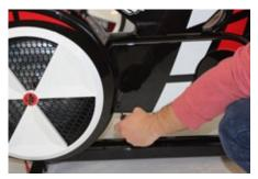
3. Use a cross head screw driver to remove the 4 x 20mm screws attaching the turbine cover on the right hand side of the bike, ensuring you hold the turbine cover whilst removing it.
