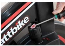
2. Use a 4mm Allen key and insert it in to the middle of the magnetic adjuster dial and unscrew the Allen headed bolt.
