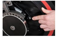
8. Remove the left hand cover and thread down the left hand crank.
