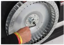
3. Remove the fan wheel. Occasionally the fan wheel can seize to the Axel. A gear puller may be required to help remove the fan wheel.
