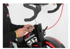
3. Use a 2.5mm Allen key to remove the screw holding the cover to the frame.
