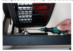
2. Using a 3mm Allen key remove all the screws attaching the turbine cover to the left hand cover
