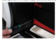
3. Use a 3mm Allen key to remove the 4x Allen headed bolts on the right hand side of the cover in the following order: 1, 2, 3, 4. Ensuring you hold the turbine cover whilst removing. SHOW NUMBERS ON PIC
