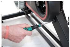
2. Use a 4mm Allen key to loosen the grub screw on the fan wheel.
