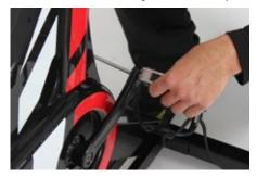
5. Use a 2.5mm Allen key to remove the two Allen headed screws holding the cover to the frame.
