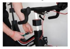
6. Continue to remove the remaining 8 shorter bolts around the cover using a 3mm Allen key.
