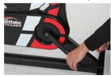
7. Use a 4mm Allen key and an 8mm spanner to remove the 2 x Allen headed bolts on the left hand side.
