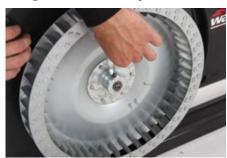
2. Use a 5mm Allen key to remove the bolt securing the fan wheel.
