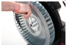
3. Using a 5mm Allen key remove the fan wheel screw.
