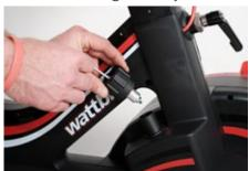
5. Use a 3mm Allen key to remove the 4 long bolts either side of the saddle and handlebar stems. **N.B Keep separate from the other screws as these are a different length.**
