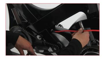
The small ridge on the block connector needs to face towards the floor and lines up with the slot in socket
