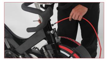
With the new cable pass it above the large pulley and between the frame of the bike
