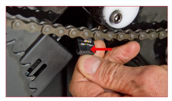
Push down from the top of the block connector. Do not force it in. Close the plastic arms to hold the plug in the socket
