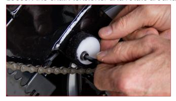
Gently pull the plastic arm attached to the socket away from the block connector at the end of the data cable. There will also be one on the other side, push this one towards the left cover
