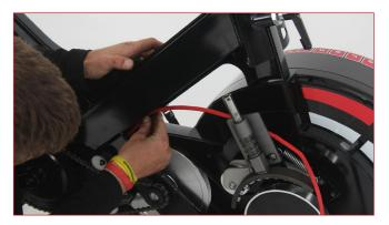
Route the cable below the screw fixing point
