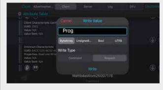
**5.** Insert the command 'prog' and press the 'Write' button at the bottom of the pop up box.
