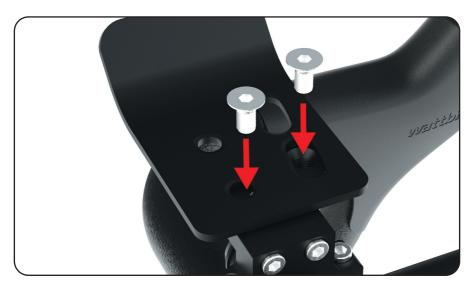
Once the mounting plate is positioned, remove the self-adhesive Velcro pad from the arm-pad and attach it to the mounting plate. Ensure to align the holes then attach the pad, ensuring that it fully covers the mounting plate.
