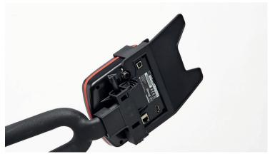
6. Reinsert the red data cable lining up the white arrow and notch guides
