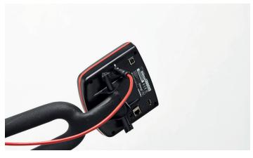
2. Undo and remove the thumb screws from the handlebars to release the monitor
