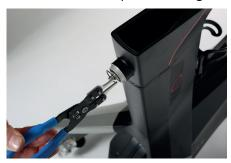
Replace the handle and unthread/unwind the threaded section of the lock lever, LL7.
