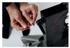
3. Remove the circlip, LL2, using a set of circlips pliers.
