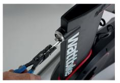
4. Replace the handle and unthread/unwind the threaded section of the Lock Lever, LL1.
