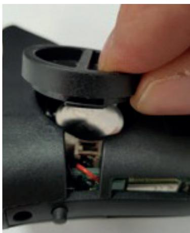
5. Remove the battery by placing a narrow flat head screw driver at the bottom of the battery (see picture below)
