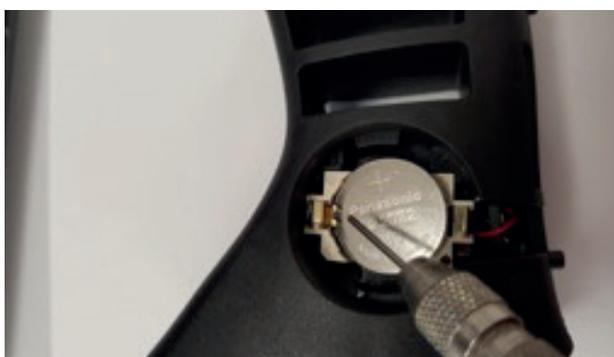
18. If you can not see the ends of the 2 brass clips they have gone under the battery and are not making a connection. Remove the battery and gently lift the 2 brass clips up so the battery can push up against them.
